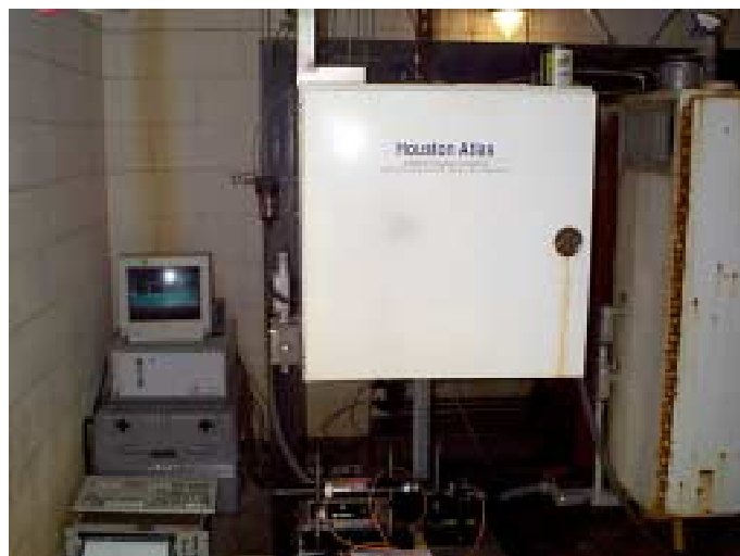
Figure 1. H 2 S Analyzer and Multi-Pass Sampling Cell Deployed Behind Houston Atlas Instrument at NCPA.
